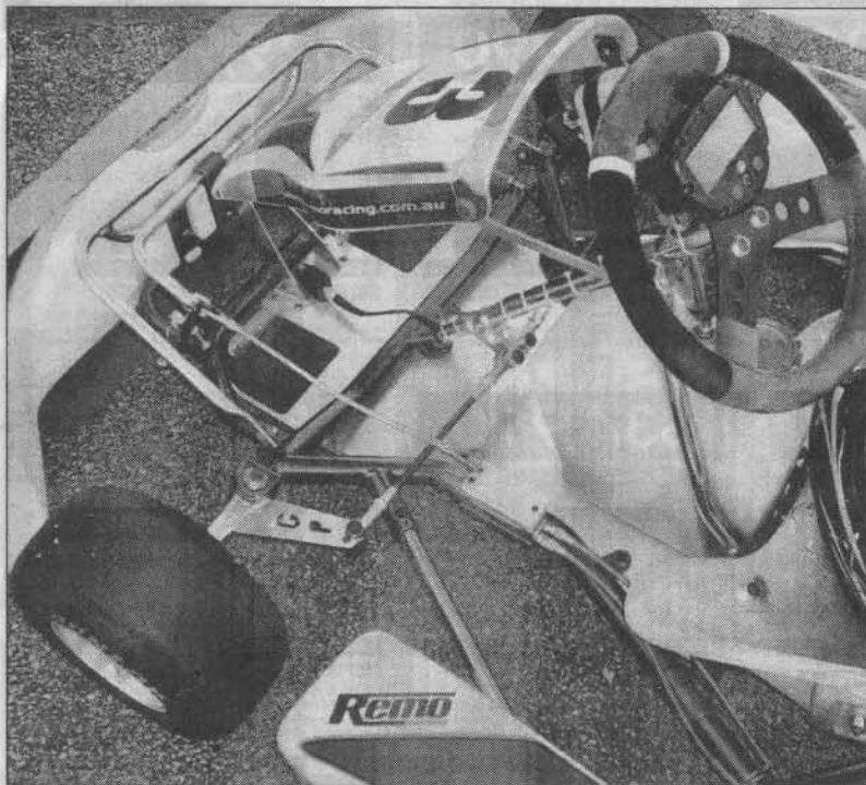
The sharp steering system also stops the inside rear wheel dragging in corners.
