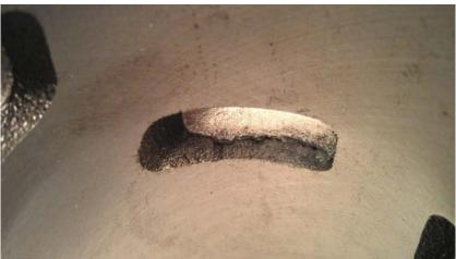
From this it can be seen that the actual port edge is both rough, in addition to positional variations, and also has a mismatch between the aluminium and the cast iron liner port where the aluminium has overflowed into the liner port
