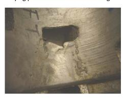
between the cylinders, particularly in the transfer ports. In the process of using the "halved" cylinder as the pattern, the cast-in cast iron liner became loose and was removed. This revealed a casting flaw (see adjacent pic) in the aluminium under the transfer port. Whilst this may have been an exception, it does show where variances may lie. It is unknown if this was a good or bad cylinder. The STRIKE cylinder provides a solution to that at a very moderate cost.
