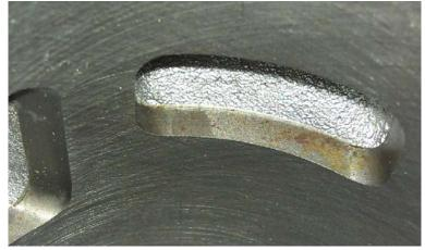
From this, it can be seen that the critical times edges of the exhaust ports and transfer ports are controlled by the accurate machining process, not by as cast edges.
