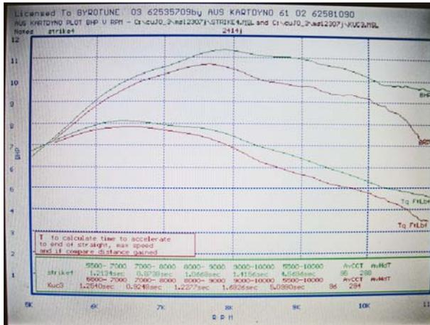
The cylinder was compared to 3 cylinders, the first one shown on the left shows the STRIKE cylinder (green line) compared to a "very average" Yamaha J cylinder (red line). The difference is very obvious.
