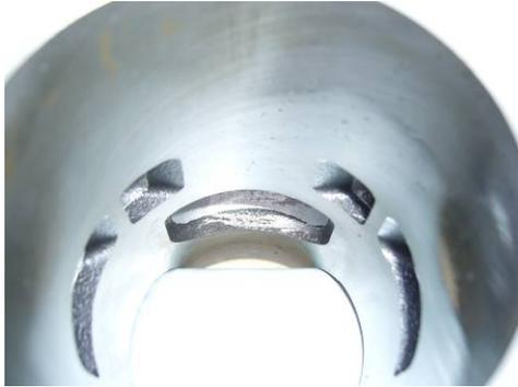
The second shows a KT100S cylinder that has had some excessive (illegal) grinding, on the base of the inlet port, presumably to clean up some surface imperfections.
