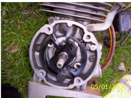
shoes is approximately equal. Finally tighten the screws to a torque of 22 - 24 Nm (16 - 18 ft lb). Both screws must be tightened. Another method of positioning the shoes is to fit a narrow 1 mm spacer made from plastic, cardboard etc) on the crankcase boss and slide the shoe assembly up to this prior to tightening. The spacer must be removed after tightening. This completes the installation of the shoe assembly.
